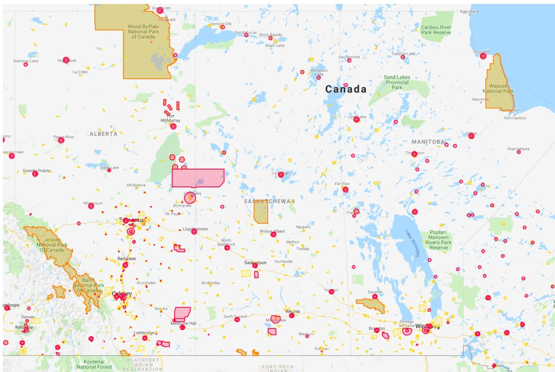
The Drone Site Selection Tool provides a graphical way for RPAS pilots to find where they can fly legally. It shows restricted, controlled and safe flying areas, and helps pilots ensure they comply with Transport Canada drone safety requirements: <https://nrc.canada.ca/en/drone-tool/>
